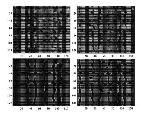
Fig.5 Microstructure evolution of  $Ni_{75}A1_{15}Ti_{10}$  aged at 1373 K+1173 K: (a) t=60 000, (b) t=63 000, (c) t=120 000, and (d) t=200 000
