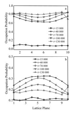
Fig.4 Variation of occupation probabilities of  $\gamma'$  phase in Ni<sub>75</sub>A1<sub>15</sub>Ti<sub>10</sub> aged at 1173 K on lattice plane: (a) Al and (b) Ti
