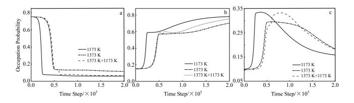
Fig.6 Variation of the occupation of different atoms at  $\beta$  site in the Ni<sub>75</sub>Al<sub>15</sub>Ti<sub>10</sub> alloy aged with different aging processes at different time: (a) Ni, (b) Al, and (c) Ti
