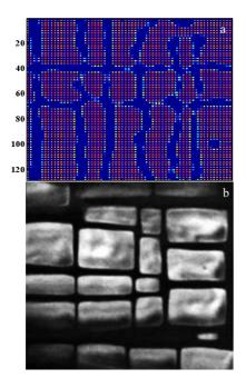
Fig.7  $\gamma'$  phase morphology obtained from simulated results (a) and experiment observation (b)
