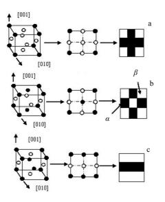
Fig.1 Ordered  $\gamma'$  phase structure and the [010] direction of 2D projection: (a) L1<sub>2</sub> phase, (b) L1<sub>0</sub> (I) phase, and (c) L1<sub>0</sub> (II) phase
