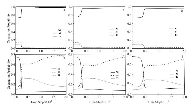
Fig.3 Variation of occupation probabilities of Ni, Al, Ti atoms at  $\alpha$  site (a, c, e) and  $\beta$  site (b, d, f) with different aging temperatures: (a, b) *T*=1173 K, (c, d) *T*=1273 K, and (e, f) *T*=1373 K
