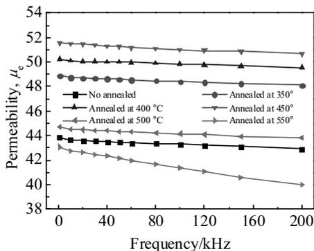
Fig.4 Permeability ( $\mu_e$ ) of the Fe<sub>95</sub>Si<sub>1</sub>B<sub>2</sub>P<sub>0.5</sub>Cu<sub>1.5</sub> magnetic powder core annealed at different temperatures for 1 h
