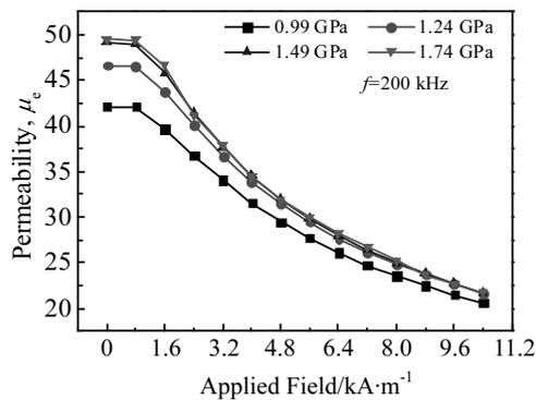
Fig.7 Curves of DC-bias property for  $\text{Fe}_{95}\text{Si}_1\text{B}_2\text{P}_{0.5}\text{Cu}_{1.5}$  magnetic powder core
