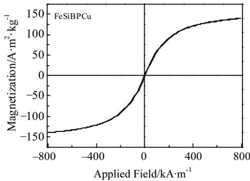
Fig.3 Magnetic hysteresis loop for the Fe<sub>95</sub>Si<sub>1</sub>B<sub>2</sub>P<sub>0.5</sub>Cu<sub>1.5</sub> alloy powders
