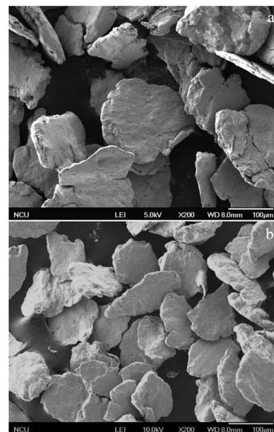
Fig.1 SEM images of  $\text{Fe}_{95}\text{Si}_1\text{B}_2\text{P}_{0.5}\text{Cu}_{1.5}$  alloy powders: (a) 75~150  $\mu\text{m}$  and (b) 45~75  $\mu\text{m}$
