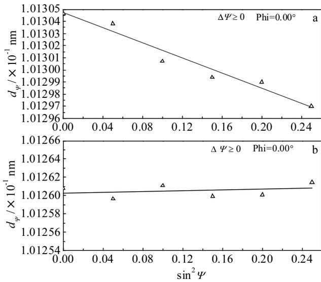
Fig.5 Plots of  $d_\psi - \sin^2\psi$  for  $\text{Fe}_{95}\text{Si}_1\text{B}_2\text{P}_{0.5}\text{Cu}_{1.5}$  magnetic powder core before (a) and after (b) annealing measured by XRD
