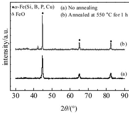
Fig.2 XRD patterns of Fe<sub>95</sub>Si<sub>1</sub>B<sub>2</sub>P<sub>0.5</sub>Cu<sub>1.5</sub> alloy powders
