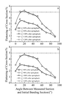
Fig.8 Section flattening of TA18 high strength tube at different relative push assistant speeds: (a) considering the variation law of CSR-*E* and (b) without considering the variation law of CSR-*E*
