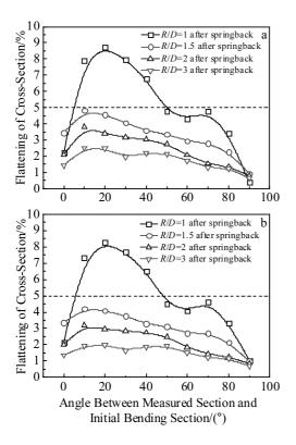
Fig.3 Section flattening of TA18 high strength tube at different *R/D*:(a) considering the variation law of CSR-*E* and (b) without considering the variation law of CSR-*E*
