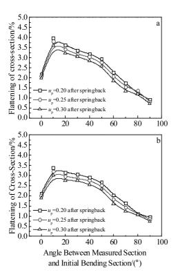
Fig.6 Section flattening of TA18 high strength tube at different friction coefficients between pressure die-tube: (a) considering the variation law of CSR-*E* and (b) without considering the variation law of CSR-*E*
