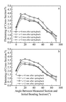
Fig.5 Section flattening of TA18 high strength tube at different mandrel extension lengths: (a) considering the variation law of CSR-*E* and (b) without considering the variation law of CSR-*E*
