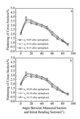
Fig.7 Section flattening of TA18 high strength tube at different friction coefficients between bending die-tube: (a) considering the variation law of CSR-*E* and (b) without considering the variation law of CSR-*E*
