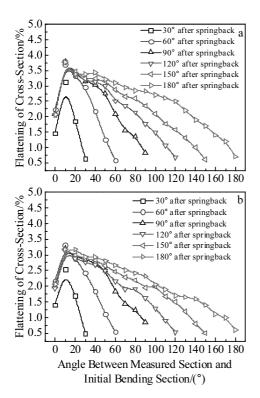
Fig.4 Section flattening of TA18 high strength tube at different bending angles: (a) considering the variation law of CSR-*E* and (b) without considering the variation law of CSR-*E*
