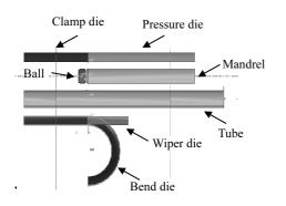
Fig.1 FE model for the NC bending of TA18 high strength tube
