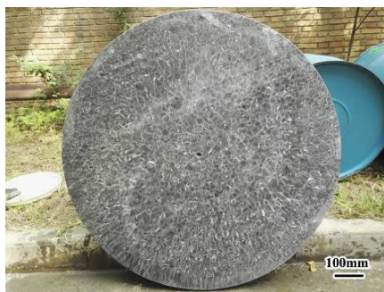
图 5 12 t 级 Ti80 合金头部低倍组织 Fig.5 Macrostructure of the 12 t ingot of Ti80 alloy at the riser
