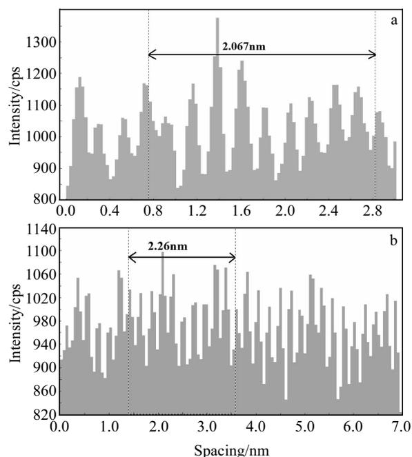
Fig.7 Interlayer spacings for the nanodiamond (111) plane (a) and hexagonal diamond (100) (b)
