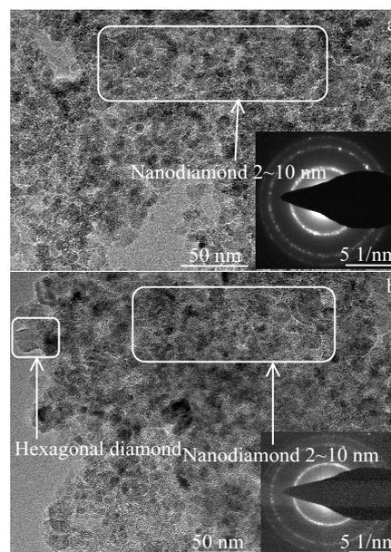
Fig.6 TEM images and SAED patterns of the nanodiamond (a) and boron-doped product (b)
