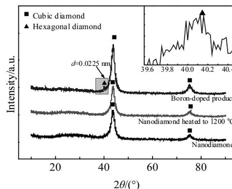
Fig.3 XRD patterns of nanodiamond, nanodiamond heated to 1200 °C, and boron-doped product
