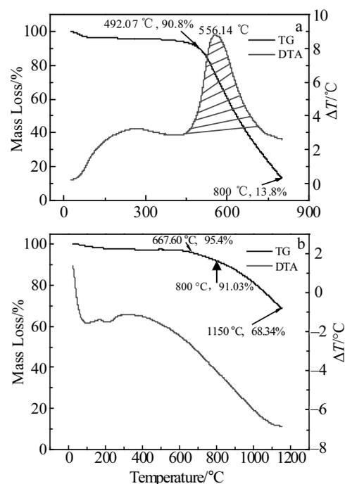
Fig.1 TG and DTA curves for nanodiamond (a) and 1:1 boron-doped product (b)
