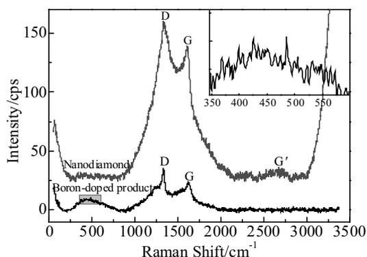
Fig.5 Raman spectra for the nanodiamond and boron-doped product
