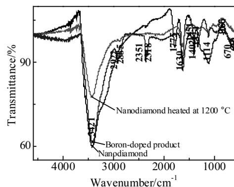
Fig.4 FTIR spectra of nanodiamond, nanodiamond heated at 1200 °C, and boron-doped product
