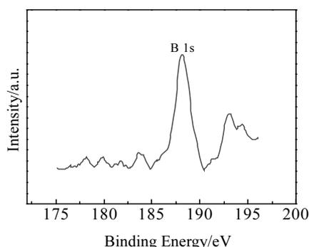
Fig.2 XPS spectrum of B 1s for boron-doped product
