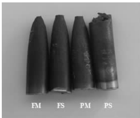
Fig.6 Macroscopical fractures during the cooling process
