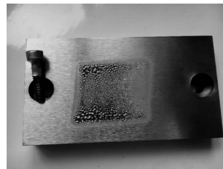
Fig.3 Surface of TZM after heating test
