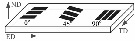
Fig.1 Schematic diagram of Mg-Zn-Ca alloy sheets sampling sites for stretched specimen (ND: normal direction, ED: extruded direction, TD: transverse direction)
