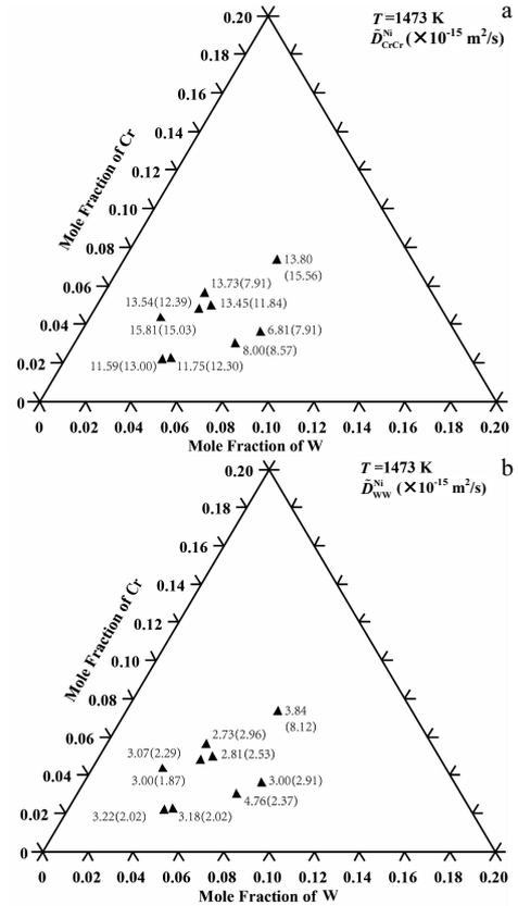
Fig.2 Comparison between the calculated main interdiffusion coefficients (numbers in brackets) and the experimental measurements: (a)  $\bar{D}_{CrCr}^{Ni}$  and (b)  $\bar{D}_{WW}^{Ni}$
