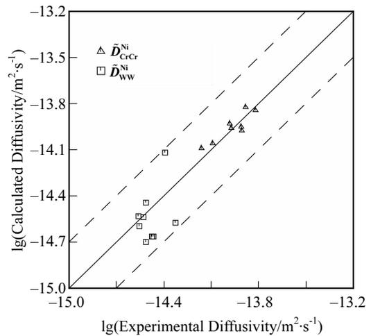
Fig.3 Comparison between the calculated main interdiffusion coefficients of the fcc Ni-Cr-W system at 1473 K and the experimental values
