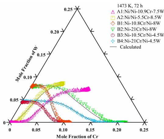
Fig.5 Comparison between the calculated and the measured diffusion paths for the six diffusion couples (A1, A2, B1, B2, B3 and B4) annealed at 1473 K for 72 h
