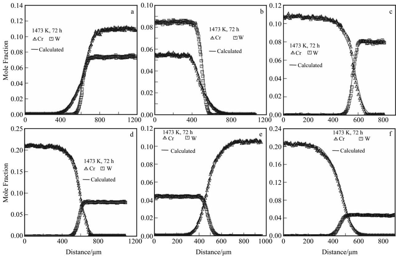
Fig.4 Model-predicted concentration profiles of six diffusion couples annealed at 1473 K for 72 h together with the corresponding experimental ones measured in the present work: (a) A1, (b) A2, (c) B1, (d) B2, (e) B3, and (f) B4
