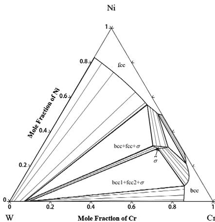
Fig.1 Calculated isothermal section at 1473 K in the Ni-Cr-W system using the thermodynamic parameters of Gustafson<sup>[20]</sup>
