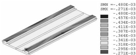
图 7 Bladder 同时打压 18 MPa 时对应的 Load-keys 间隙 Fig.7 Load-keys gap opened with all bladders pressurized at the same time up to 18 MPa
