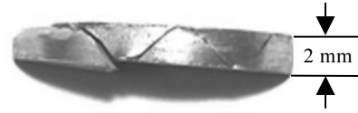
图 7 T=150\text{ }^\circ\text{C} 、 \dot{\epsilon}=3500\text{ s}^{-1} 时试样的侧面图 Fig.7 Profile of sample at T=150\text{ }^\circ\text{C} and \dot{\epsilon}=3500\text{ s}^{-1}
