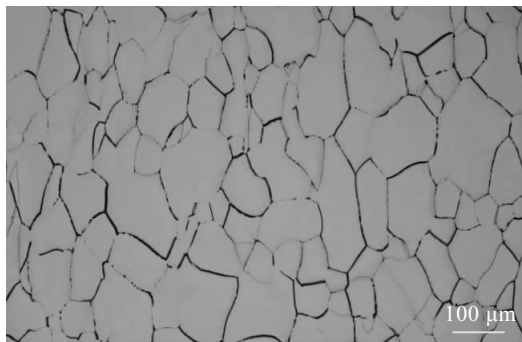
图 1 TB18 合金棒材固溶 ( 840\text{ }^\circ\text{C}\times 2\text{ h} ) 水冷后金相显微组织 Fig.1 Metallograph of TB18 Ti alloy with solution treatment ( 840\text{ }^\circ\text{C}\times 2\text{ h} + \text{water quenching} )
