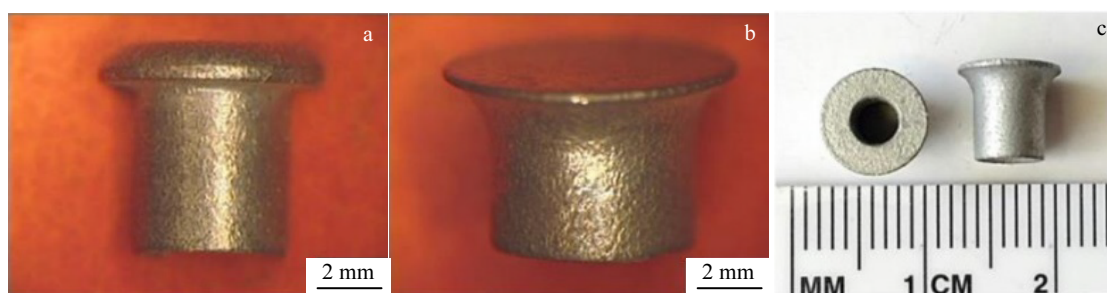
Fig.3 Appearances of different rivet head shapes: (a) domed head self-piercing rivet [24] , (b) countersunk head self-piercing rivet [24] , and (c) hollow tubular rivet [27]
