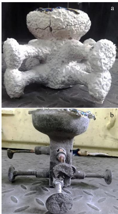
Fig.7 Valve casting with (a) and without (b) the ceramic shell mold
