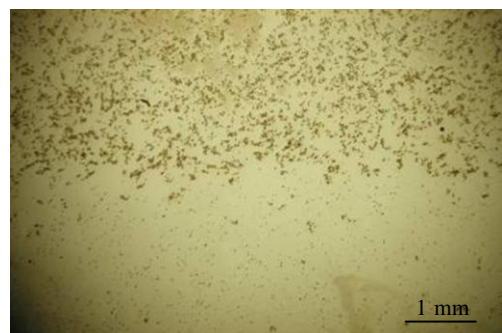
图 5 旋转磁场带芯坩埚中夹杂物宏观分布 Fig.5 Macroscopic distribution of inclusions with rotating magnetic field [28]
