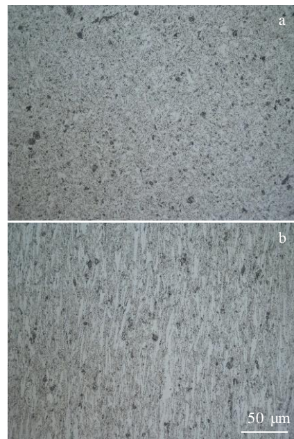
图 9 挤压比 4:1 下构型复合材料热处理后金相组织 Fig.9 OM microstructures of configuration composite after heat treatment under extrusion ratio of 4:1: (a) vertical extrusion direction and (b) parallel extrusion direction
