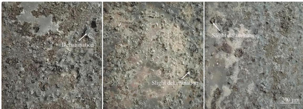
Fig.7 EXCO morphologies of Al-7.88Zn-2.05Mg-1.70Cu-0.19Er alloys after peak-aging (a), over-aging (b), and double-aging (c) treatments
