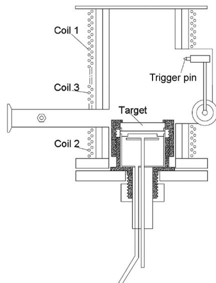
Fig.14 Schematic diagram of arc source device with zero point of magnetic field component on vertical cathode target surface<sup>[40,58-62]</sup>
