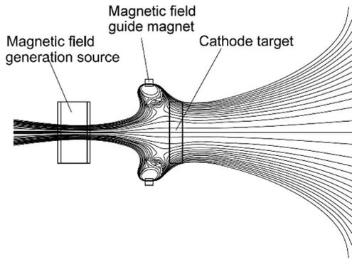
Fig.20 Schematic diagram of constrained magnetic arc source<sup>[70-71]</sup>
