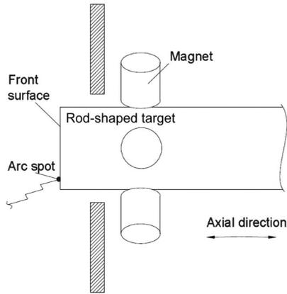
Fig.7 Schematic diagram of arc source structure with magnets on cathode side<sup>[39]</sup>
