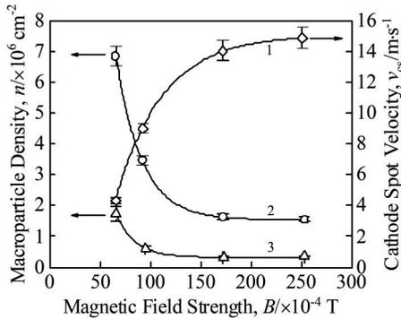
Fig.9 Macroparticle densities on target surface after exposure for 0.5 min under anode potential (line 2) and under pulsed negative bias (line 3) at different magnetic fields; relationship between cathode spot velocity and magnetic field strength (line 1)<sup>[45]</sup>
