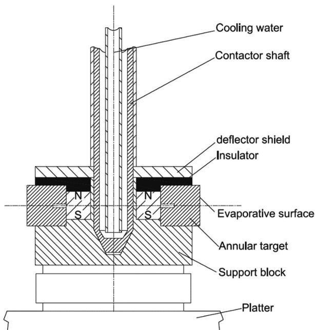
Fig.16 Schematic diagram of annular target arc source structure<sup>[61]</sup>
