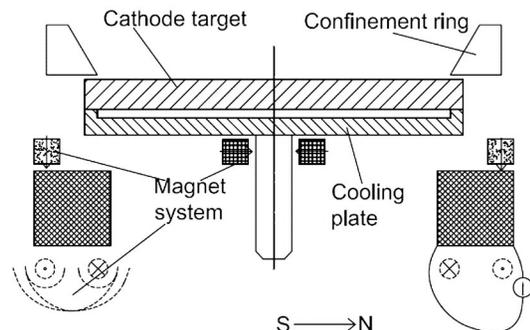
Fig.11 Amelioration of magnetic field layout of plane target with dominant horizontal magnetic field component<sup>[52]</sup>
