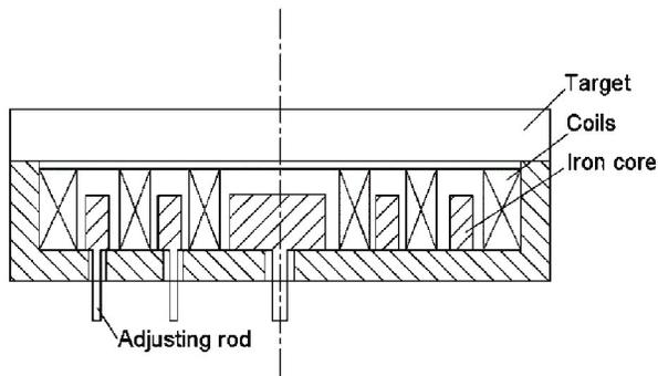
Fig.13 Schematic diagram of magnetic field structure of arc source for composite target<sup>[57]</sup>
