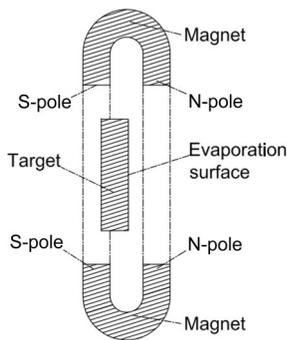
Fig.5 Schematic diagram of arc source with relatively small changes in magnetic field direction and intensity due to target evaporation
