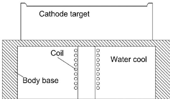
Fig.4 Schematic diagram of arc source with electromagnetic dynamic control on arc spot movement<sup>[32]</sup>
