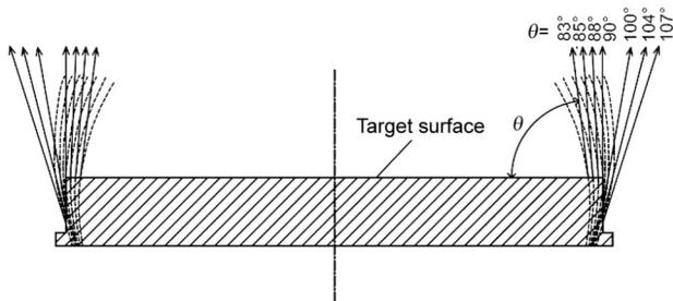
Fig.1 Angles formed by discharge surface and magnetic field of arc evaporation source<sup>[28]</sup>
