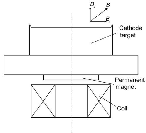
Fig.2 Schematic diagram of arc source with simple magnetic field structure<sup>[31]</sup>
