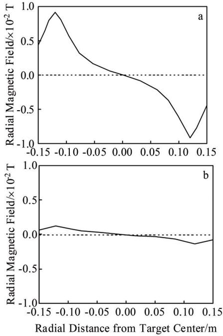
Fig.15 Comparison of horizontal component magnetic fields without (a) and with (b) coil 3<sup>[56,60]</sup>
