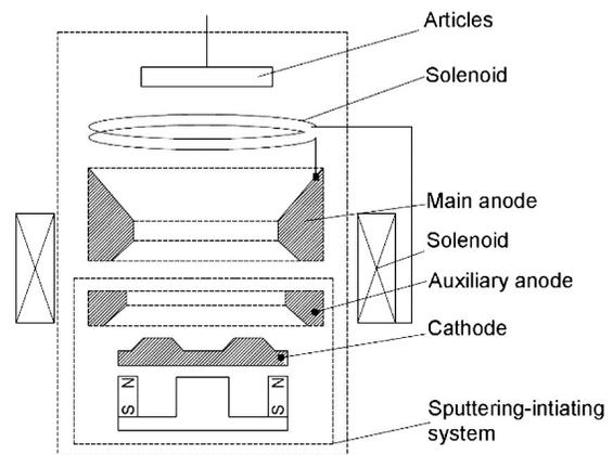
Fig.22 Schematic diagram of magnetically controlled arc striking pulse arc source<sup>[78]</sup>
