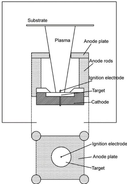
Fig.23 Schematic diagram of pulse arc source with ignition electrode in the middle of the target<sup>[79]</sup>
