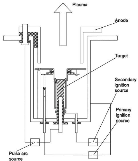
Fig.21 Schematic diagram of multi-stage trigger pulse arc source<sup>[77]</sup>
