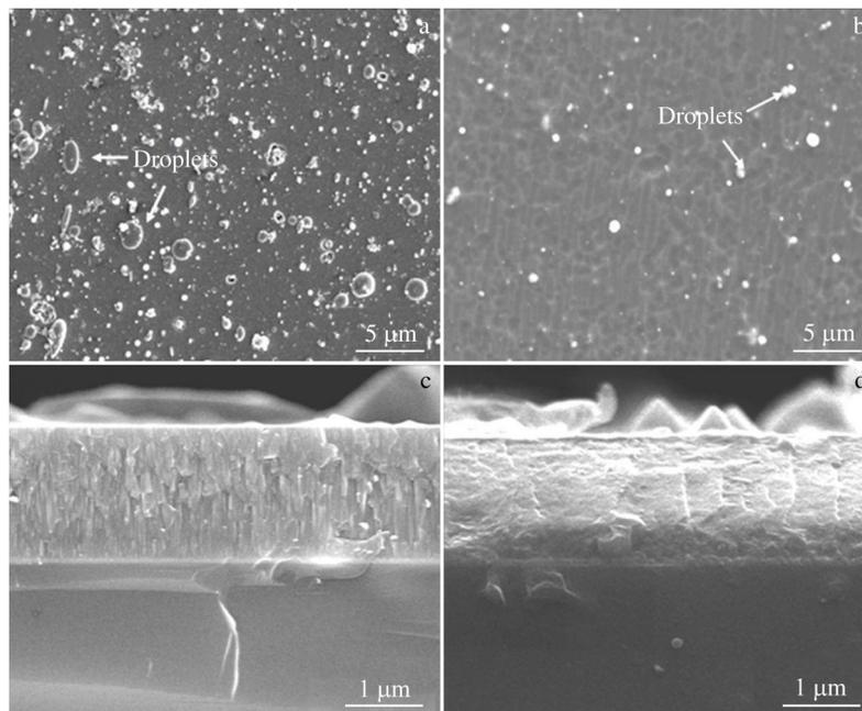
Fig.24 SEM images of surface (a–b) and cross-section (c–d) of nitride coatings deposited by conventional arc (a, c) and splitting arc (b, d)<sup>[84]</sup>
