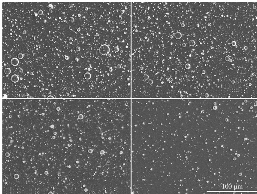
Fig.8 SEM morphologies of macroparticles on target surfaces of TiN films under different transverse magnetic fields: (a) 0 T, (b) 0.01 T, (c) 0.02 T, and (d) 0.03 T<sup>[44]</sup>
