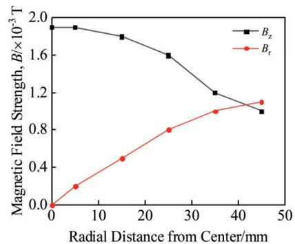
Fig.3 Typical value of magnetic field of single-structural permanent magnetic structure
