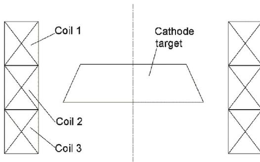
Fig.18 Schematic diagram of DC arc source coil structure<sup>[21,46]</sup>
