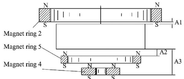
Fig.17 Schematic diagram of arc source with multi-magnetic ring structure<sup>[64]</sup>
