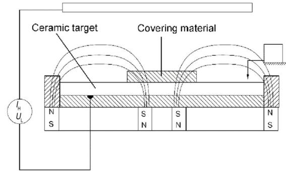
Fig.10 Schematic diagram of magnetic field layout of plane target with dominant horizontal magnetic field component<sup>[48]</sup>
