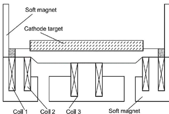
Fig.19 Schematic diagram of magnetic shielding structure of arc source<sup>[68]</sup>
