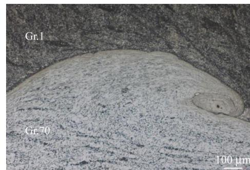
Fig.8 OM image of interface structure of titanium-steel composite plate after process 4
