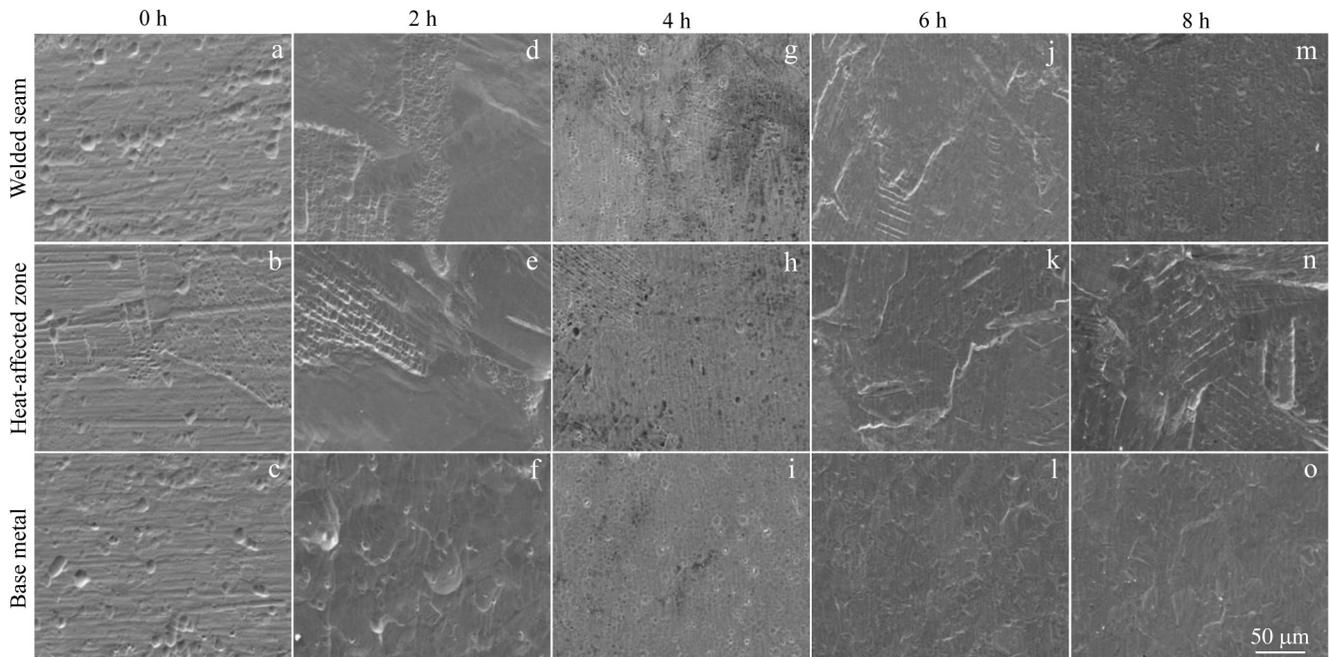
Fig.3 SEM morphologies of welded seam (a, d, g, j, m), heat-affected zone (b, e, h, k, n), and base metal (c, f, i, l, o) areas after oxidation at 550 °C for 0 h (a–c), 2 h (d–f), 4 h (g–i), 6 h (j–l), and 8 h (m–o)
