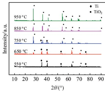
Fig.7 XRD patterns of white products on welded joint after oxidation at different temperatures for 4 h
