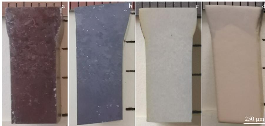
Fig.4 Appearances of welded joints after oxidation at 650 °C (a), 750 °C (b), 850 °C (c), and 950 °C (d) for 4 h
