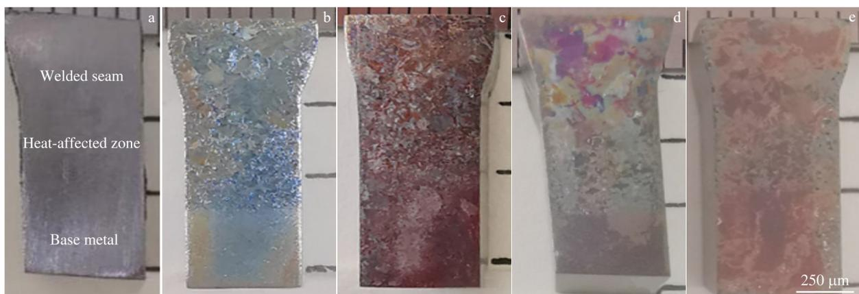
Fig.1 Appearances of welded joints after high temperature oxidation at 550 °C for 0 h (a), 2 h (b), 4 h (c), 6 h (d), and 8 h (e)
