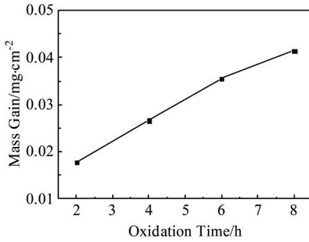
Fig.2 Mass gain of welded joint after oxidation at 550 °C for different durations
