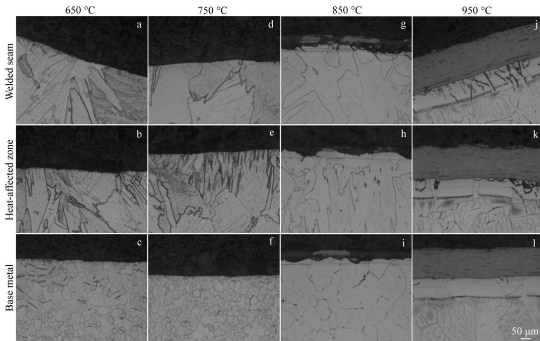
Fig.9 Microstructures of welded seam (a, d, g, j), heat-affected zone (b, e, h, k), and base metal (c, f, i, l) areas after oxidation at 650 °C (a–c), 750 °C (d–f), 850 °C (g–i), and 950 °C (j–l) for 4 h
