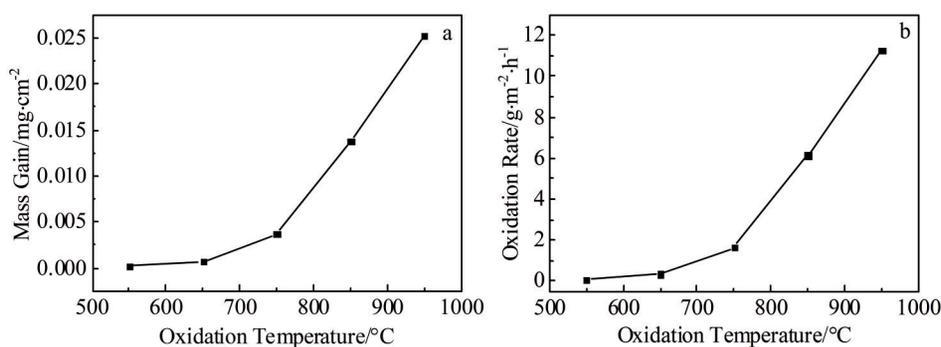
Fig.5 Mass gain (a) and oxidation rate (b) of welded joints after oxidation at different temperatures for 4 h
