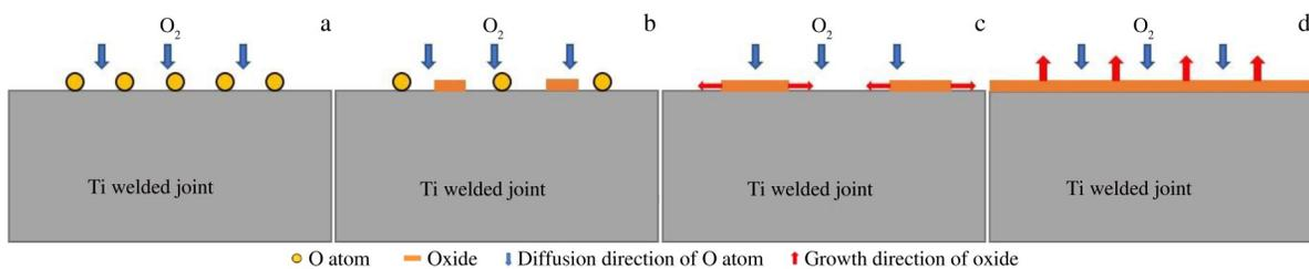
Fig.10 Schematic diagrams of oxidation film formation on surface of welded joint: (a) O<sub>2</sub> absorption on surface; (b) preferential nucleation in defective zone; (c) lateral oxide growth; (d) oxidation film growth and thickening
