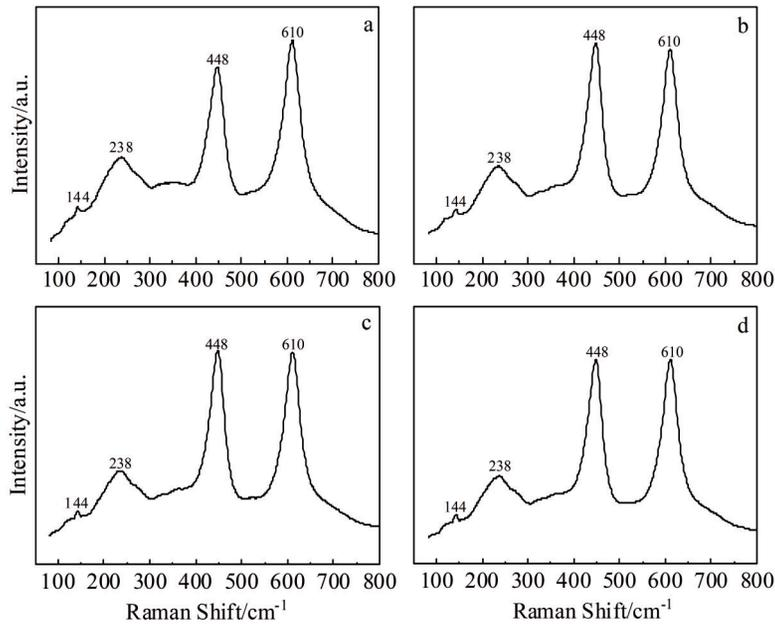
Fig.8 Raman spectra of welded joints after oxidation at different temperatures for 4 h: (a) 650 °C, (b) 750 °C, (c) 850 °C, and (d) 950 °C
