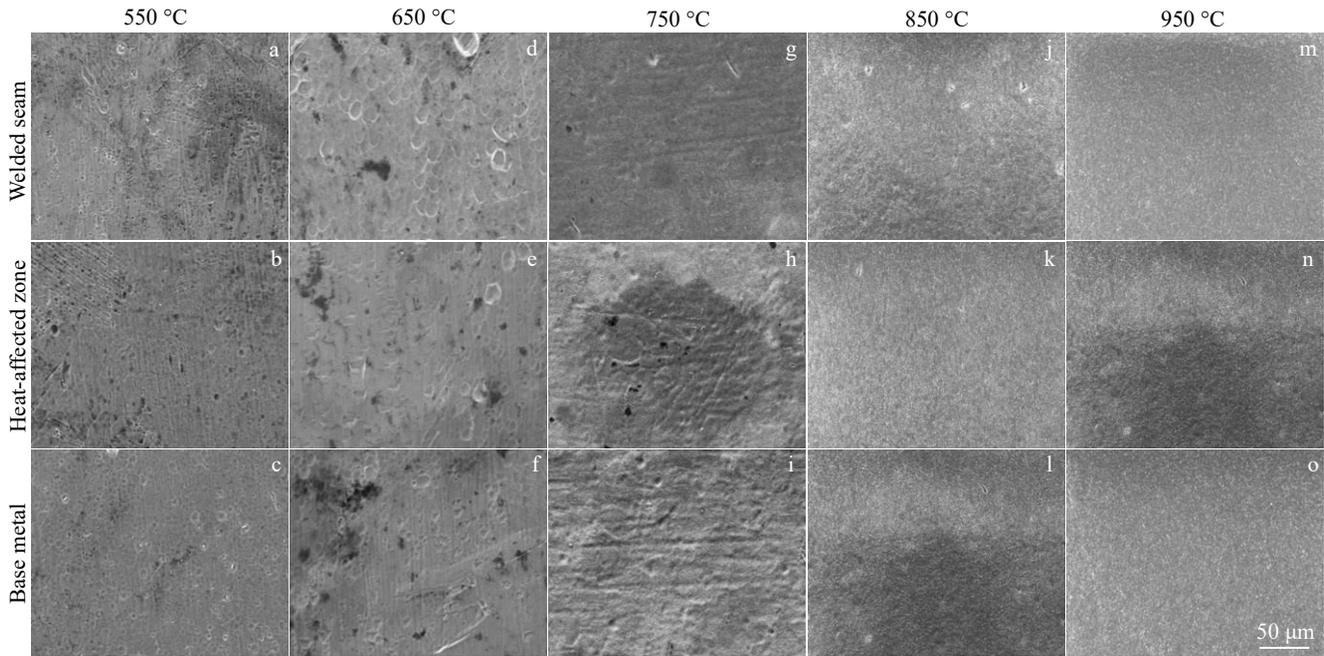
Fig.6 SEM morphologies of welded seam (a, d, g, j, m), heat-affected zone (b, e, h, k, n), and base metal (c, f, i, l, o) areas after oxidation at 550 °C (a–c), 650 °C (d–f), 750 °C (g–i), 850 °C (j–l), and 950 °C (m–o) for 4 h
