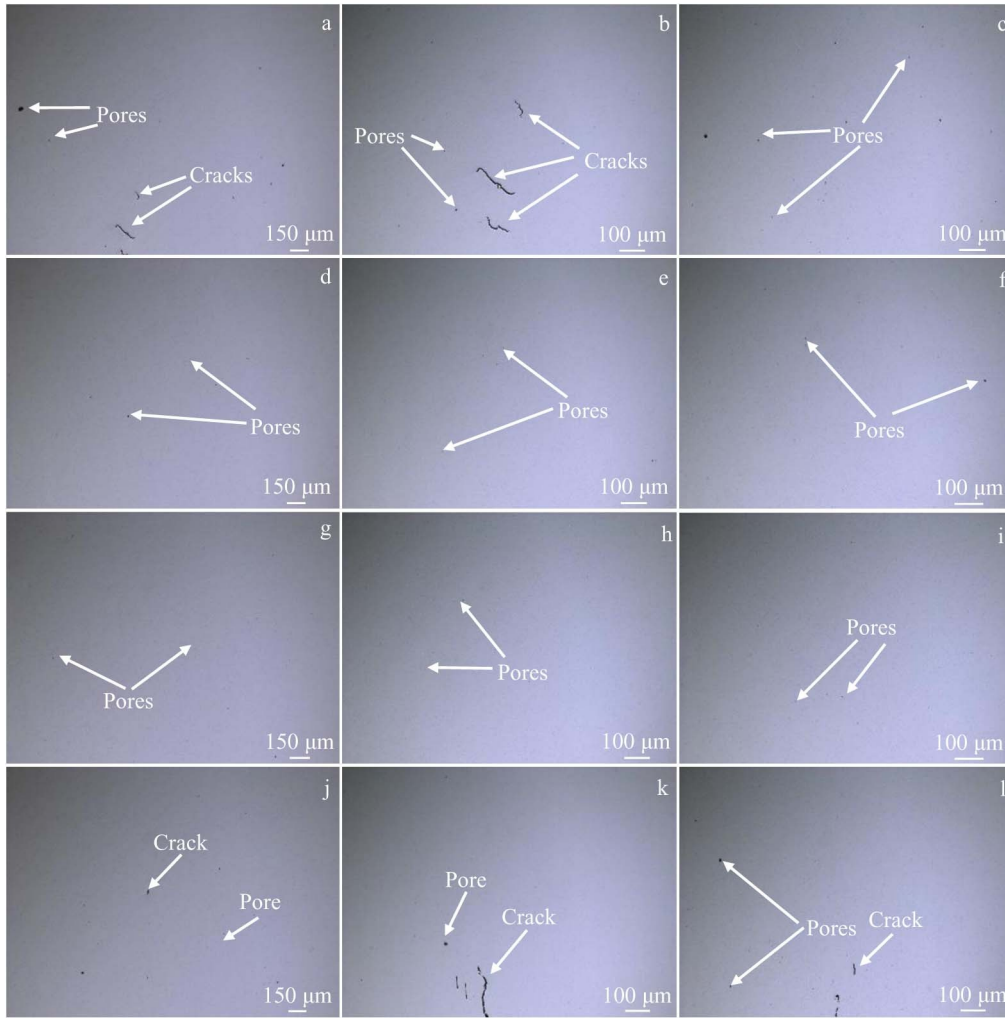
Fig.5 OM images of as-fabricated ZGH451 specimens obtained after various treatments: (a–c) LPBF, (d–f) HIP, (g–i) HIP+HT, and (j–l) HT
