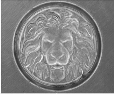
Fig.8 Appearance of HEMG specimen after thermoforming
