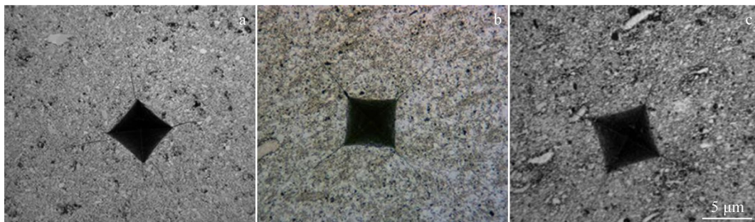
Fig.10 Vickers indentation patterns of MoSi 2 material (a), twice-coated MoSi 2 @Nb material (b), and once-coated MoSi 2 @Nb material (c)
