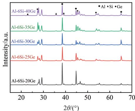
Fig.2 XRD patterns of Al-6Si-*y*Ge filler metals
