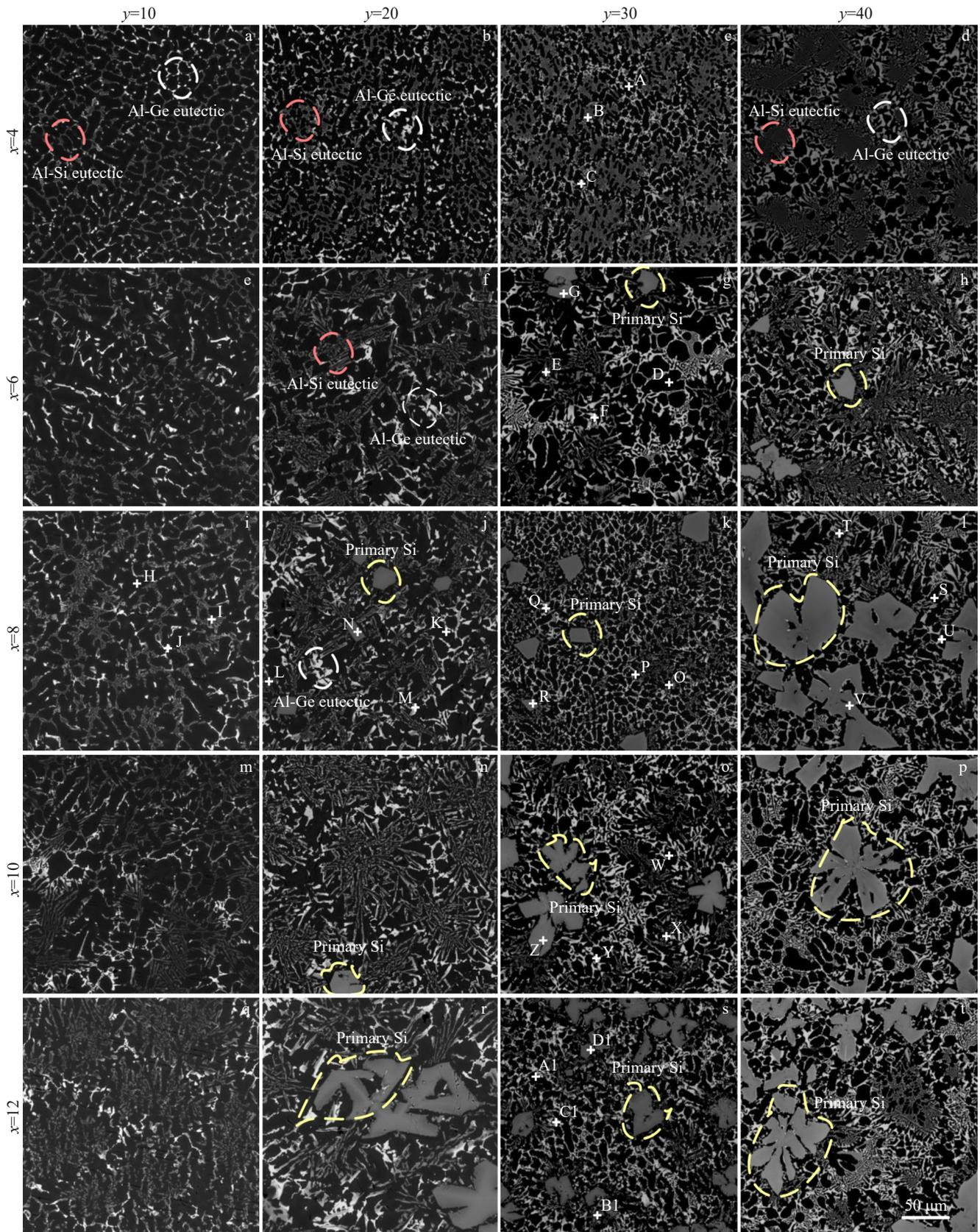
Fig.1 Microstructures of different Al-xSi-yGe filler metals
