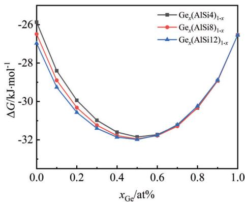
Fig.5 Influence of Ge addition on free energy of Al-Si binary system
