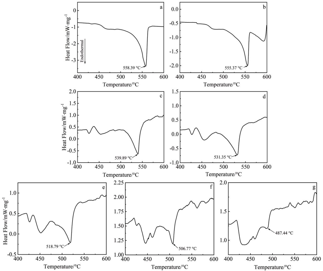
Fig.3 DSC curves of Al-xSi-yGe filler metals: (a) Al-8Si-10Ge; (b) Al-8Si-15Ge; (c) Al-8Si-20Ge; (d) Al-8Si-25Ge; (e) Al-8Si-30Ge; (f) Al-8Si-35Ge; (g) Al-8Si-40Ge
