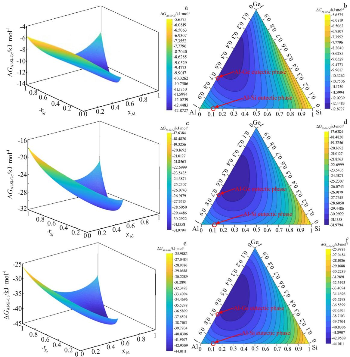
Fig.4 3D (a, c, e) and 2D (b, d, f) free energy contour maps of Al-Si-Ge ternary alloy system at different temperatures: (a–b) 25 °C; (c–d) 400 °C; (e–f) 600 °C
