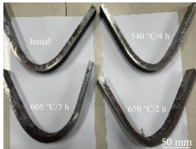
Fig.11 Internal bending results of zirconium-titanium-steel composite plate at different states
