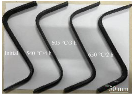
Fig.10 S-type bending results of zirconium-titanium complex at different states
