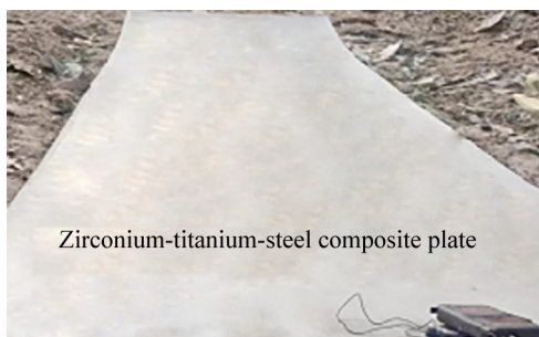
Fig.8 Appearance of zirconium-titanium-steel composite plate after explosive welding
