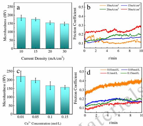
Fig. 5. Vickers hardness and friction coefficient curves of coatings under different current densities and  $\text{Cu}^{2+}$  concentrations.
