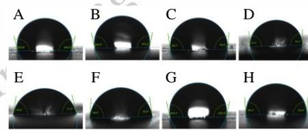
Fig. 6. Water CA of coatings under different current densities and  $\text{Cu}^{2+}$  concentrations.
