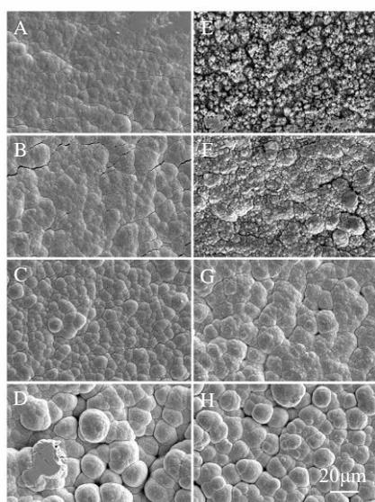
Fig. 1. Micromorphology of Cu-Ni coating under different current densities and  $\text{Cu}^{2+}$  concentrations.
