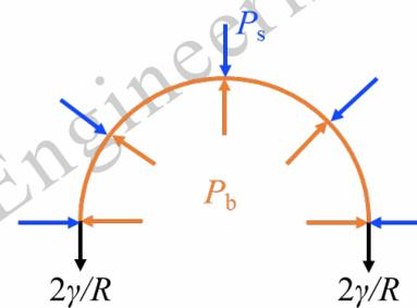
Fig.1 The force analysis of the fission gas bubble
