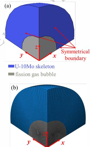
Fig.2 Diagrams of (a) the FE model containing the equivalent solid of fission gas bubble and the U-10Mo skeleton (b) the mesh grid
