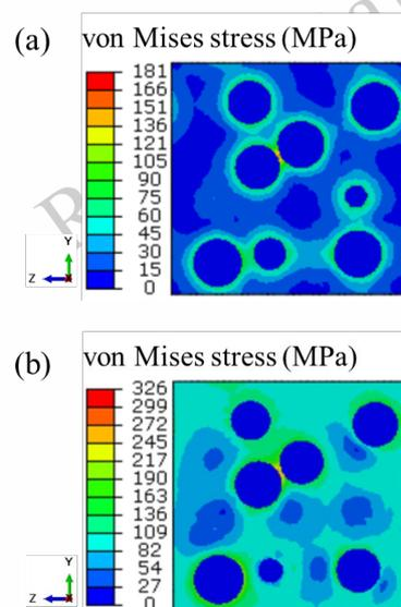
Fig.6 The contour plots of the von Mises stress on the cross section in the  $x$  direction of the RVE (a) before loading and (b) after loading
