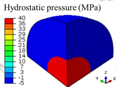
Fig.3 The contour plots of the hydrostatic pressure in FE model with the pressured fission gas bubble before applying the external pressure
