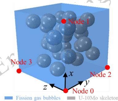
Fig.5 The RVE of irradiated U-10Mo fuels with randomly distributed FGBs
