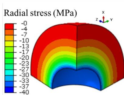
Fig.11 The contour plots of radial stress of the surrounding fuel skeleton before the application of external pressure
