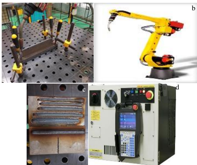
Fig.1 Appearances of welding table (a), FANUC Arc Mate 100iC Robotic machine (b), welded SS (c), and robot controller (d)
