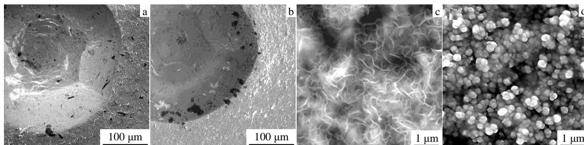
Fig.4 SEM indent morphologies of the TLM alloy samples and their surfaces tested with a home-used scotch tape: (a, c) TLM, 120 °C, heat treated; (b, d) TLM, 150 °C, heat treated
