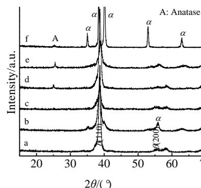
Fig.2 XRD patterns of the hydrothermally treated and the heat treated samples: (a) TLM, 120 °C; (b) TLM, 120 °C, heat treated; (c) TLM, 135 °C; (d) TLM, 150 °C; (e) TLM, 150 °C, heat treated; (f) Ti, 150 °C
