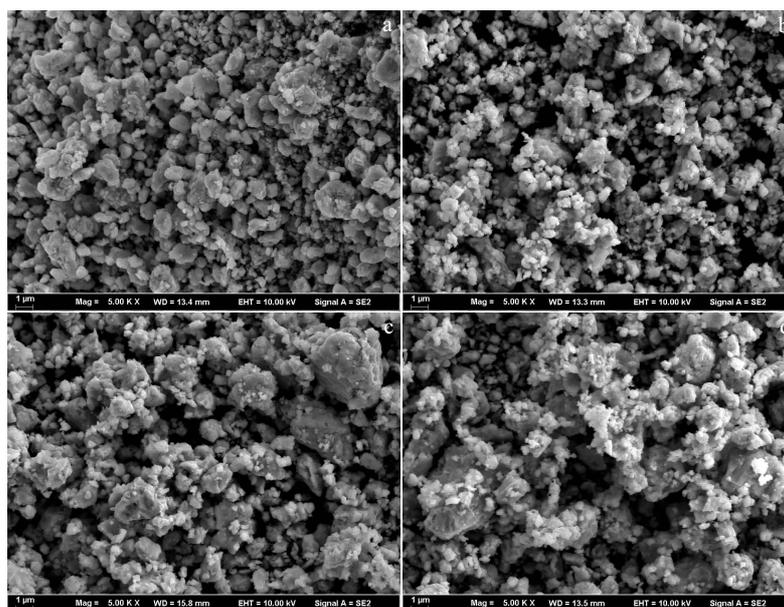
Fig.8 Wear debris of (TiC+TiB)/Ti6Al4V composites with volume fraction of 15% under different loads: (a) 5 N, (b) 10 N, (c) 15 N, and (d) 20 N
