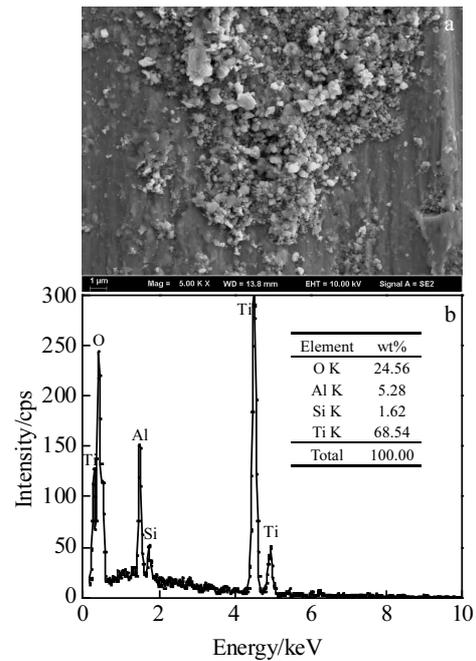
Fig.7 Worn surface morphologies (a) and corresponding EDS analysis (b) for (TiC+TiB)/Ti6Al4V composite with volume fraction of 15% under the load of 20 N
