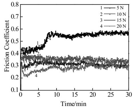
Fig.5 Friction coefficient curves of composites with volume fraction of 15% as a function of sliding time under different loads
