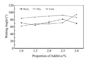
Fig.2 Wetting angle between Ag and SnO<sub>2</sub>
