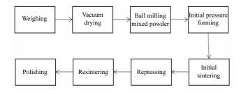
Fig.1 Manufacturing process of contact materials
