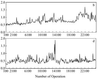
Fig.3 Contact resistance of Ag-SnO<sub>2</sub> contact materials doped with Bi<sub>2</sub>O<sub>3</sub> of different particle sizes: (a) 200 nm, (b) 500 nm, (c) 1 μm, and (d) 10 μm
