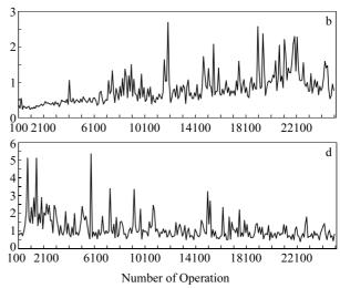
Fig.5 Contact resistance of Ag-SnO<sub>2</sub> contact materials doped with CeO<sub>2</sub> of different particle sizes: (a) 200 nm, (b) 500 nm, (c) 1 μm, and (d) 10 μm
