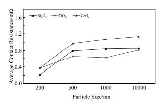
Fig.6 Average contact resistance of Ag-SnO<sub>2</sub> contact materials
