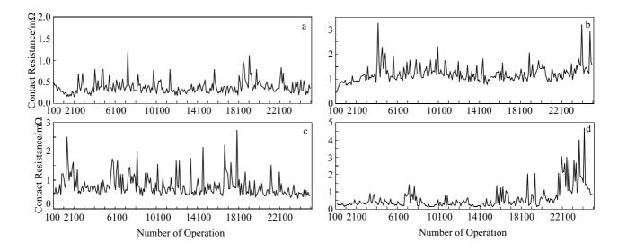
Fig.4 Contact resistance of Ag-SnO<sub>2</sub> contact materials doped with TiO<sub>2</sub> of different particle sizes: (a) 200 nm, (b) 500 nm, (c) 1 μm, and (d) 10 μm
