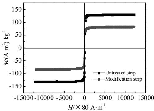
Fig.8 Hysteresis loops of amorphous alloy strips
