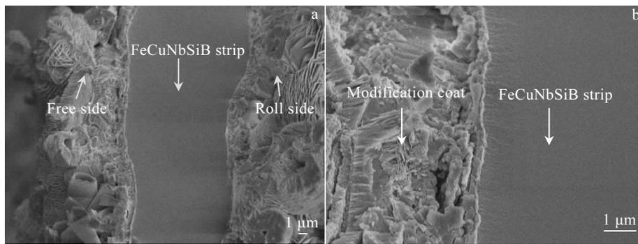
Fig.4 Microstructures of the strips before (a) and after (b) surface chemical modification
