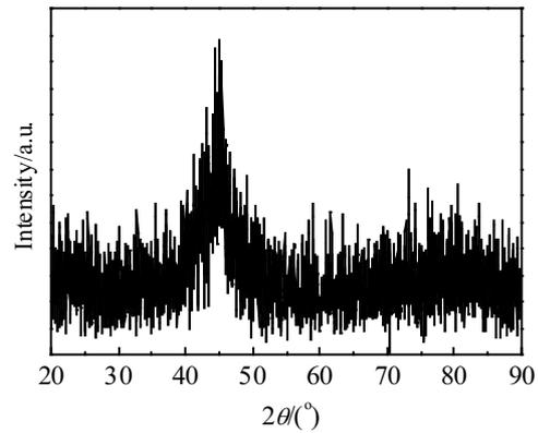
Fig.1 XRD pattern of FeCuNbSiB amorphous alloy strip
