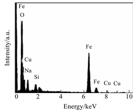
Fig.5 EDS spectrum of the strip conversion coat
