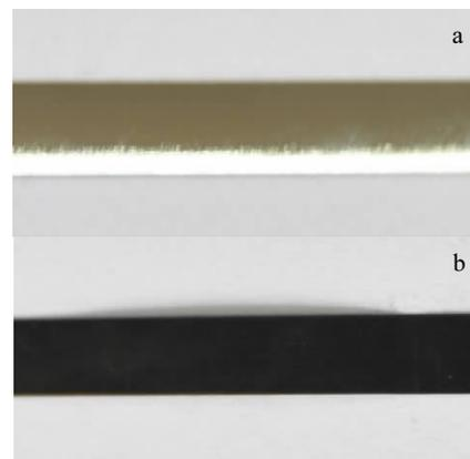
Fig.2 Photos of strips before (a) and after (b) surface chemical modification
