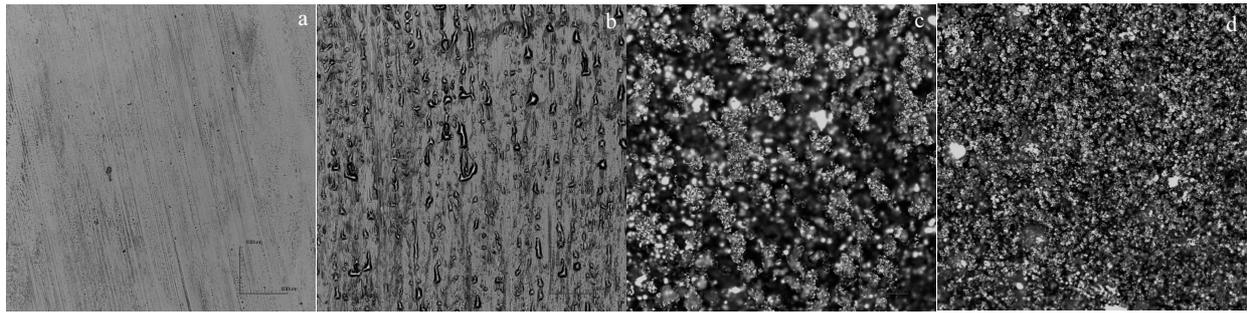
Fig.3 Surface morphologies of the strips before and after surface chemical modification: (a) free side of untreated strip; (b) roll side of untreated strip; (c) free side of modification strip; (d) roll side of modification strip
