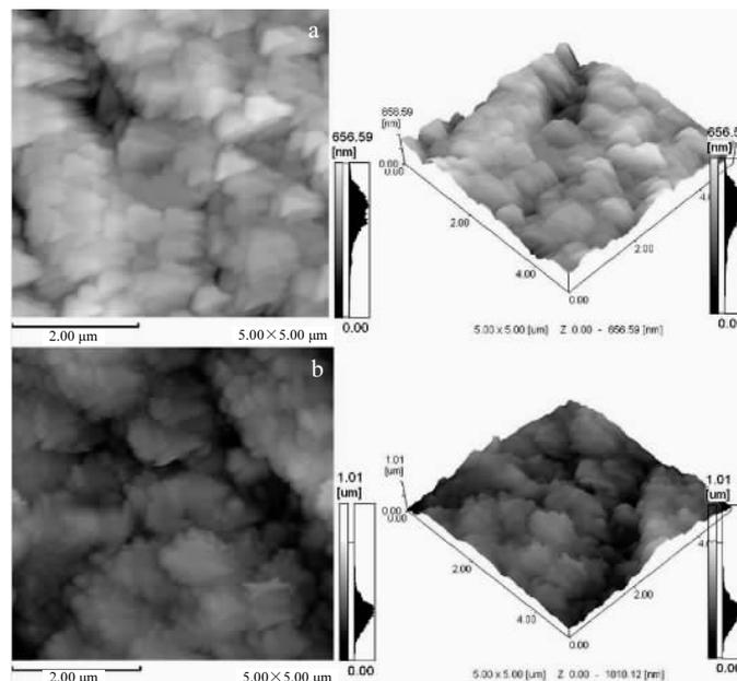
Fig.4 AFM surface images of the  $In_xGa_{1-x}N$  (a) and Mg-doped  $In_xGa_{1-x}N$  (b) thin films
