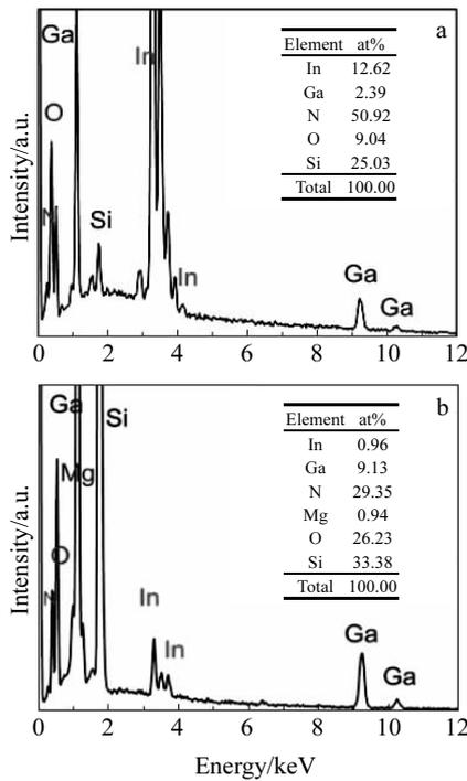
Fig.3 EDS spectra of the  $In_xGa_{1-x}N$  (a) and Mg-doped  $In_xGa_{1-x}N$  (b) thin films
