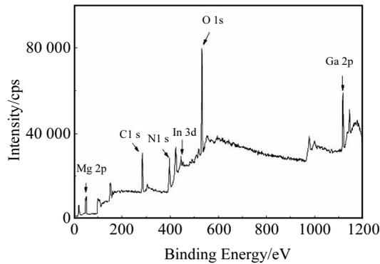
Fig.5 XPS spectrum of Mg-doped  $\text{In}_x\text{Ga}_{1-x}\text{N}$  thin films
