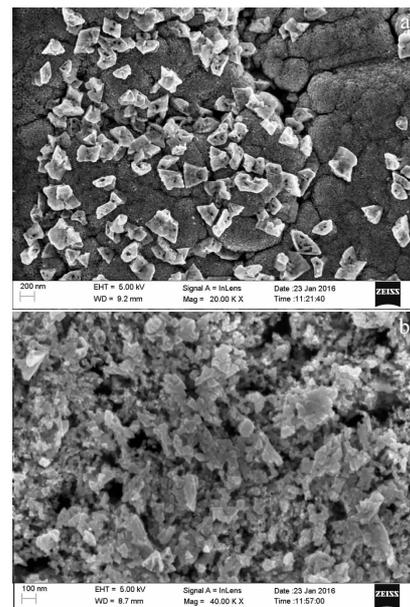
Fig.2 SEM images of the  $\text{In}_x\text{Ga}_{1-x}\text{N}$  (a) and Mg-doped  $\text{In}_x\text{Ga}_{1-x}\text{N}$  (b) thin films
