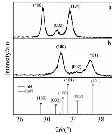
Fig.1 XRD patterns of  $\text{In}_x\text{Ga}_{1-x}\text{N}$  (a) and Mg-doped  $\text{In}_x\text{Ga}_{1-x}\text{N}$  (b) thin films
