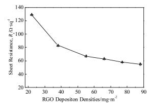
Fig.6 R<sub>s</sub> versus rGO deposition density of AgNWs/rGO films
