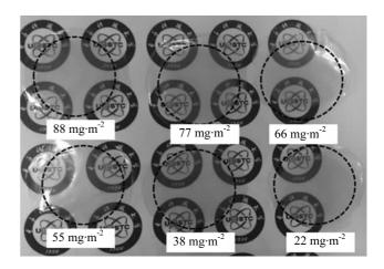
Fig.3 Photos of AgNWs/rGO films with 220 mg·m<sup>-2</sup> AgNWs and different deposition densities of rGO
