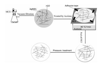
Fig.1 Schematic of fabrication process of AgNWs/rGO-MCE film
