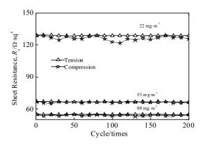
Fig.8 R<sub>s</sub> of AgNWs-rGO films after cycles of folding up
