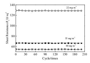
Fig.7 R<sub>s</sub> of AgNWs-rGO films after taping test
