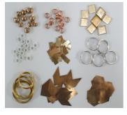
Fig.4 Morphology of the preformed filler metal
