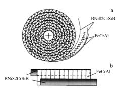
Fig.2 Schematic diagram of assembling brazing sample: (a) top view and (b) position of the brazing filler metal<sup>[13]</sup>
