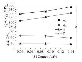
Fig.2 Tensile properties of each alloy
