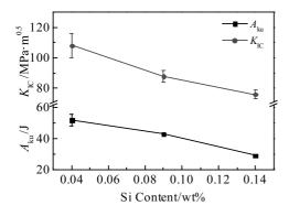
Fig.4 Effect of Si content on impact energy and  $K_{IC}$
