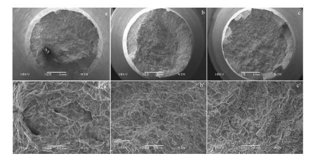
Fig.6 Tensile fracture morphologies of three alloys at RT: (a, a') alloy A, (b, b') alloy B, and (c, c') alloy C
