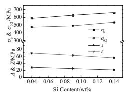
Fig.5 High temperature tensile properties of each alloy at 500 °C
