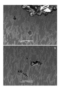
Fig.9 Typical microstructure of the fracture of alloy A (a) and alloy B (b)
