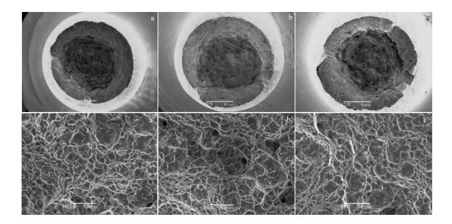
Fig.7 Tensile fracture morphologies of three alloys at 500 °C: (a, a') alloy A, (b, b') alloy B, and (c, c') alloy C
