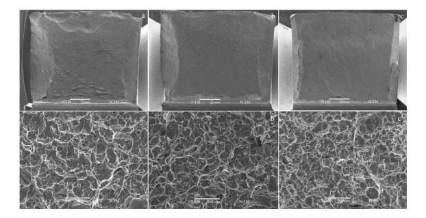
Fig.8 Impact toughness fracture morphologies of three alloys at RT: (a, a') alloy A, (b, b') alloy B, and (c, c') alloy C
