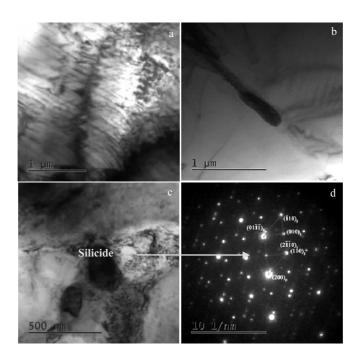
Fig.12 TEM images of alloy C: (a, b) dislocations, (c) grain boundaries and phase boundaries, and (d) SAED pattern of silicide of (Ti, Zr)<sub>x</sub>Si<sub>y</sub>
