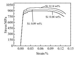
Fig.3 Effect of Si content on tensile properties at room temperature
