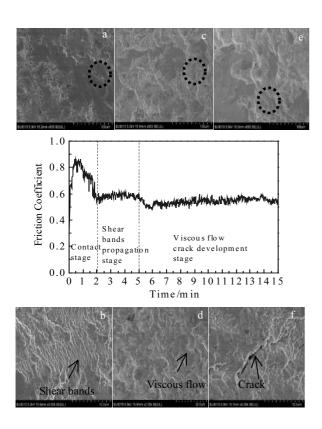
Fig. 3 Friction coefficient value and worn surface morphologies of composite coating with 20 wt% ZrO<sub>2</sub> at 50 N load:
