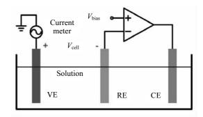
Fig.1 Diagram of the three-electrode system
