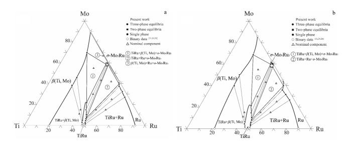
Fig.4 Experimentally determined isothermal section of Mo-Ru-Ti system at 1100 °C (a) and 1300 °C (b)
