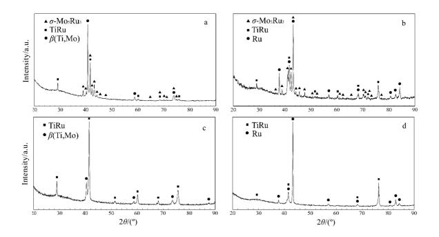
Fig.3 XRD patterns of ternary Mo-Ru-Ti alloys: (a)  $Mo_{55}Ru_{30}Ti_{15}$  alloy annealed at 1300 °C for 15 d, (b)  $Mo_{42}Ru_{51}Ti_7$  alloy annealed at 1100 °C for 50 d, (c)  $Mo_{15}Ru_{30}Ti_{46}$  alloy annealed at 1300 °C for 15 d, and (d)  $Mo_{15}Ru_{60}Ti_{25}$  alloy annealed at 1100 °C for 50 d
