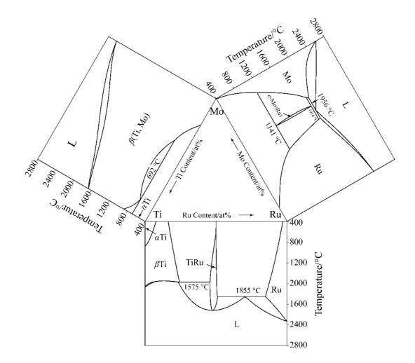
Fig.1 Binary phase diagrams constituting the Mo-Ru-Ti ternary system<sup>[11,20,26]</sup>
