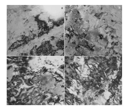
Fig.6 Microstructures of the pure Zr cold-rolled with 10% (a, b) and 20% (c, d) reduction after isochronal annealing at different temperatures for 60 min: (a, c) 473 K and (b, d) 673 K
