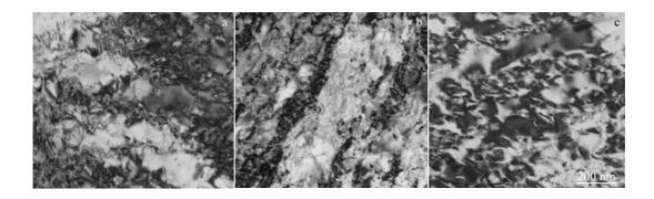
Fig.5 Microstructures of cold-rolled pure zirconium with different deformation reductions: (a) 10%, (b) 20%, and (c) 40%
