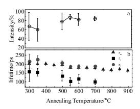
Fig.4 Intensity of the long lifetime component (a) and short lifetime, mean lifetime, long lifetime of pure zirconium cold-rolled with 20% reduction during isochronal annealing (b)
