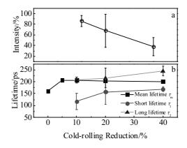
Fig.2 Intensity of long lifetime (a) and positron lifetime (b) as a function of the cold-rolling reduction for pure zirconium
