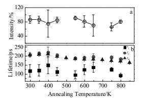
Fig.3 Intensity of the long lifetime component (a) and short lifetime, mean lifetime, long lifetime of pure zirconium cold-rolled with 10% reduction during isochronal annealing (b)
