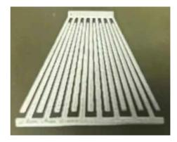
Fig.6 TIDT manufactured by screen printing on PZT
