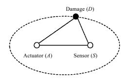
Fig.8 Schematic diagram of ellipse positioning
