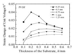
Fig.5 Unit voltage strain for different electrode widths and substrate (PVDF) thickness
