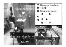
Fig.9 Photograph of the damage imaging experiment
