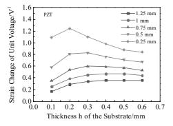
Fig.4 Unit voltage strain for different electrode widths and substrate (PZT) thickness
