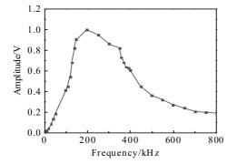
Fig.7 Normalized amplitude of the five-peak wave excited by TIDT at different excitation frequencies
