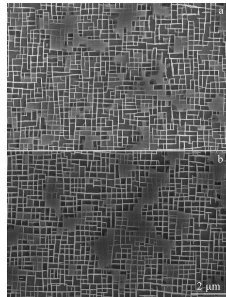
Fig.2 FSEM images of dendrite regions of D1 (a) and D2 (b) alloys
