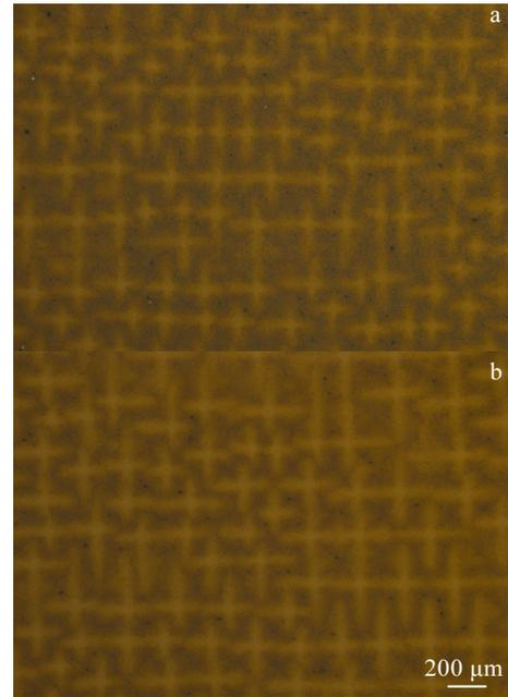
Fig.1 OM images of dendrite structure in D1 (a) and D2 (b) alloys
