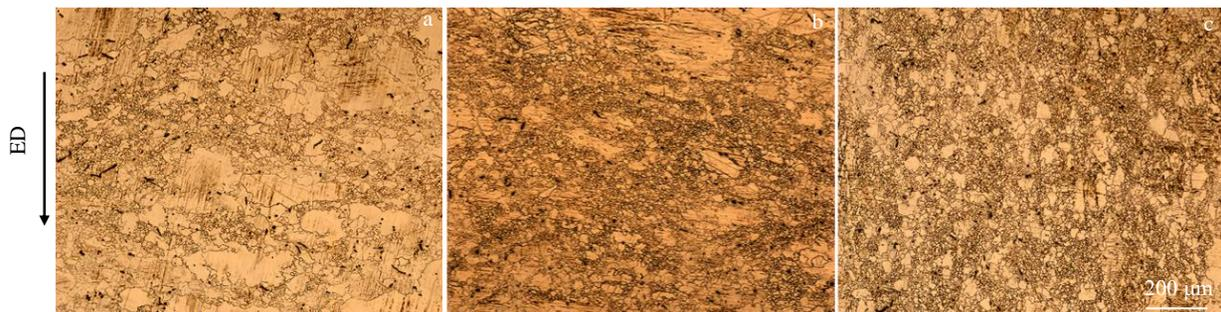
Fig.4 OM images of AZ31 Mg alloys after 1 pass (a), 2 passes (b), and 3 passes (c) of CEE-AEC process
