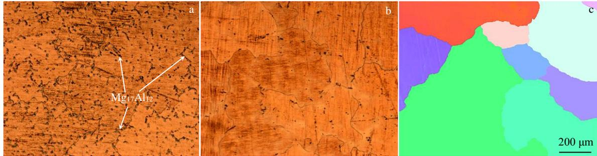
Fig.3 OM images (a, b) and EBSD inverse pole figure map (c) of as-cast (a) and homogenized (b, c) AZ31 Mg alloys
