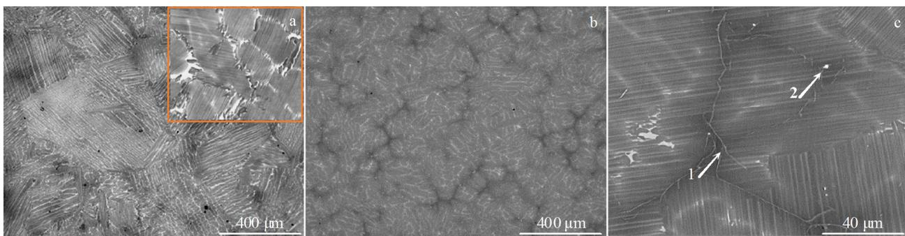
Fig.1 SEM images of initial microstructures of TWC (a) and TWC-BY (b, c) alloys
