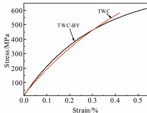
Fig.3 Room temperature stress-strain curves of alloys
