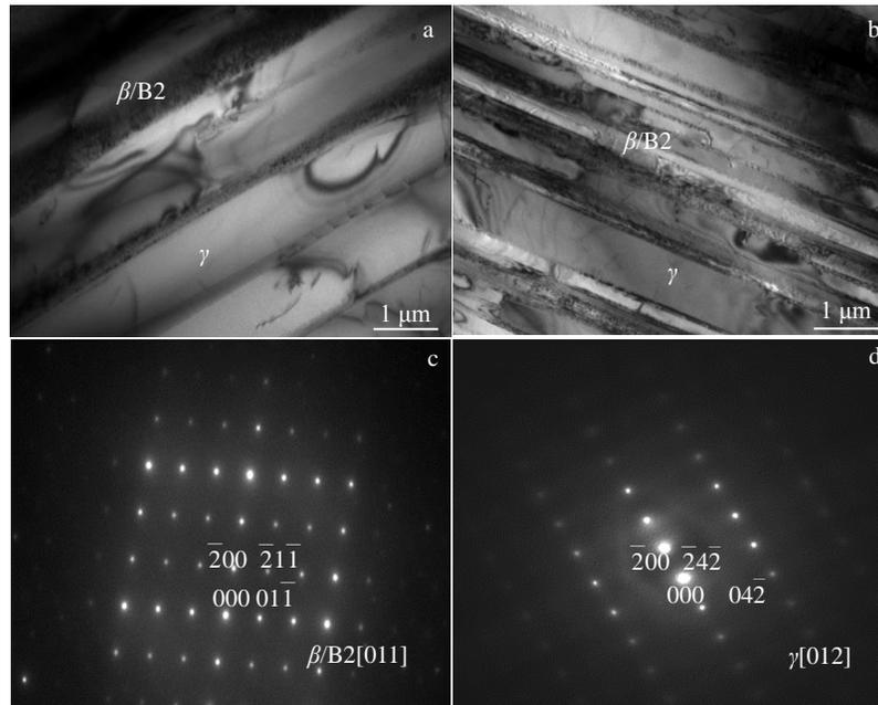
Fig.2 TEM images of lamellar microstructures of as-cast TWC (a) and TWC-BY (b) alloys; selected area electron diffraction patterns of  $\beta/\text{B}2$  phase (c) and  $\gamma$  phase (d)
