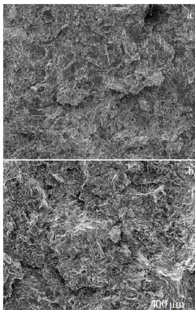
Fig.4 Tensile fracture morphologies at room temperature of TWC (a) and TWC-BY (b) alloys
