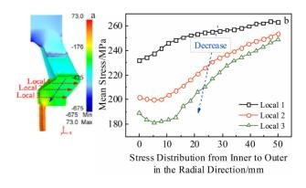
Fig.8 Mean stress distribution in welding chamber (a) and change of mean stress in the diameter direction at different locations (b)
