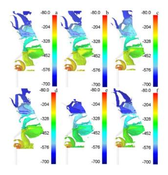
Fig.11 Iso-surface of mean stress at different billet preheating temperatures: (a)  $T_0=380$  °C, (b)  $T_0=390$  °C, (c)  $T_0=400$  °C, (d)  $T_0=410$  °C, (e)  $T_0=420$  °C, and (f)  $T_0=430$  °C
