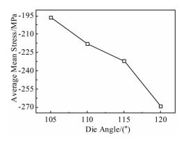
Fig.14 Effect of die angle on the average mean stress in the welding chamber
