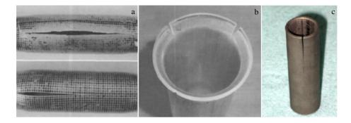
Fig.1 Cracking of the welding line of the pipe formed by the porthole extrusion method in bulging process<sup>[3]</sup> (a), extension process<sup>[3]</sup> (b), and push bending process<sup>[4]</sup> (c)
