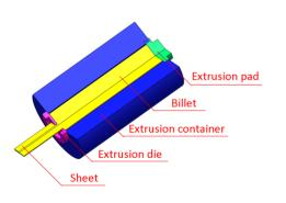
Fig.3 Geometry model for AZ91 plate extrusion process
