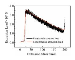
Fig.5 Comparison of extrusion load between the simulated and experimental results
