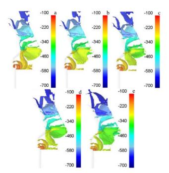
Fig.9 Iso-surface of mean stress in the welding chamber at different extrusion speeds: (a) v=2 mm/s, (b) v=4 mm/s, (c) v=6 mm/s, (d) v=8 mm/s, and (e) v=10 mm/s
