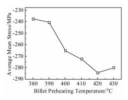
Fig.12 Effect of billet preheating temperature on the average mean stress in welding chamber
