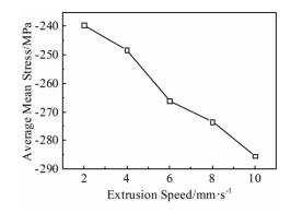
Fig.10 Effect of extrusion speed on the average mean stress in the welding chamber
