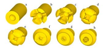
Fig.6 Metal flowing behavior in the extrusion process: (a) step 30, (b) step 70, (c) step 100, (d) step 150, (e) step 190, (f) step 220, (g) step 260, and (h) step 290
