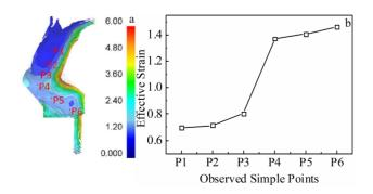
Fig.7 Effective strain distribution (a) and values (b) of the separated metal in the extrusion process of corner porthole die
