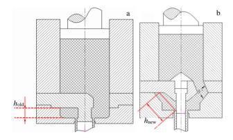
Fig.2 Present pothole extrusion method: (a) traditional extrusion and (b) welding chamber with angle
