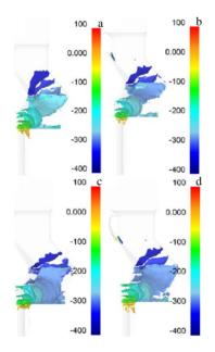
Fig.13 Iso-surface of mean stress at different die angles: (a)  $\beta$ =105°, (b)  $\beta$ =110°, (c)  $\beta$ =105°, and (d)  $\beta$ =120°
