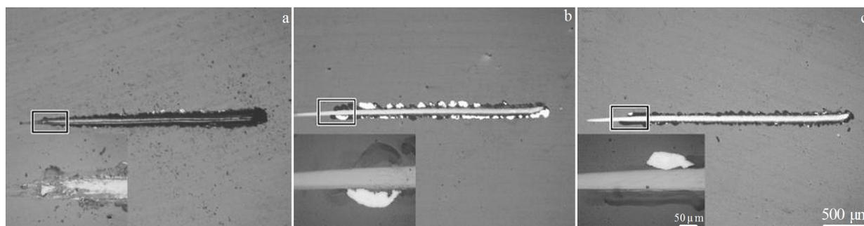
Fig.4 Scratch track morphologies of TiN films deposited by dcMS (a), HPPMS (b), and MPPMS (c)
