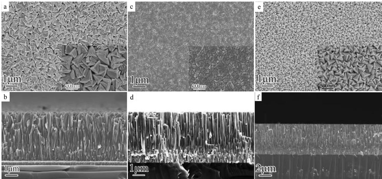
Fig.3 Surface and cross-sectional SEM micrographs of TiN films deposited by dcMS (a, b), HPPMS (c, d), and MPPMS (e, f)
