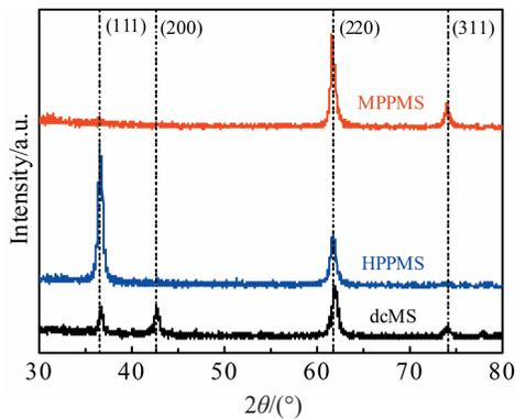
Fig.2 XRD patterns of TiN films deposited by dcMS, HPPMS and MPPMS
