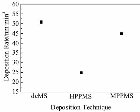
Fig.1 Average deposition rates of TiN films deposited by dcMS, HPPMS and MPPMS
