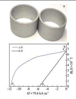
Fig.5 Optical photographs of the ring-shaped magnet (a) and magnetic properties of the RSM (b)
