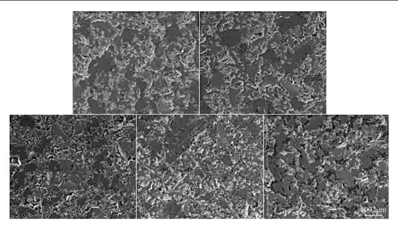
Fig.2 Surface morphologies and structures of bonded magnets with different binder contents: (a) 1wt%, (b) 2wt%, (c) 3wt%, (d) 4wt%, and (e) 5wt%
