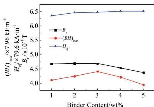
Fig.3 Curves of the magnetic properties of samples 1~5
