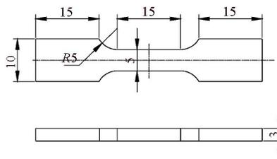
Fig.1 Tensile specimen structure drawing
