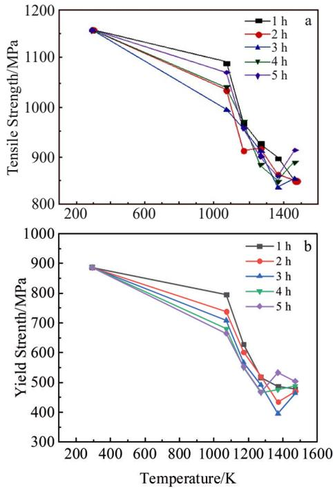
Fig.7 Tensile strength (a) and yield strength (b) of test steels after solution treatment at different temperatures
