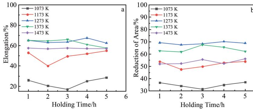
Fig.10 Elongation (a) and reduction of area (b) of test steels after solution treatment at different temperatures for different time
