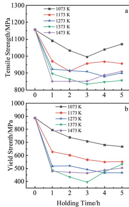
Fig.9 Tensile strength (a) and yield strength (b) of test steels after solution treatment at different temperatures for different time
