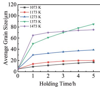
Fig.6 Effect of holding time on average grain size of test steels
