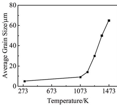
Fig.5 Grain size of test steels after holding at different temperatures for 1 h
