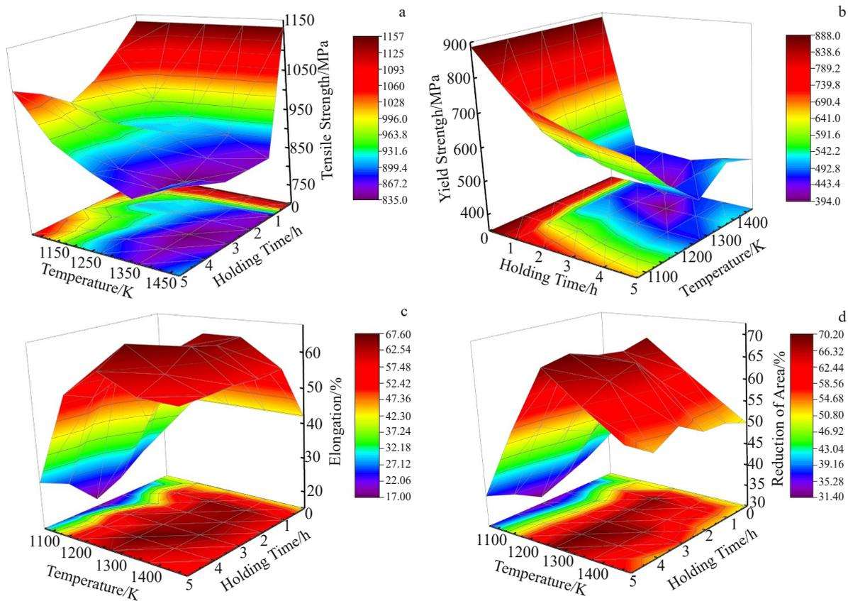
Fig.11 Combined effect of solution time and temperature on tensile strength (a), yield strength (b), elongation (c) and reduction of area (d)
