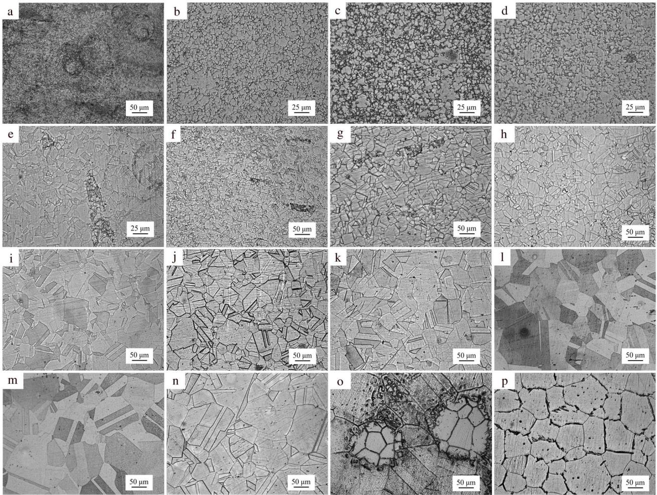
Fig.4 Microscopic structures of test steel solution treated under different conditions: (a) untreated; (b, c, d) 800 °C; (e, f, g) 900 °C; (h, i, j) 1000 °C; (k, l, m) 1100 °C; (n, o, p) 1200 °C; (b, e, h, k, n) 1 h; (c, f, i, l, o) 3 h; (d, g, j, m, p) 5 h
