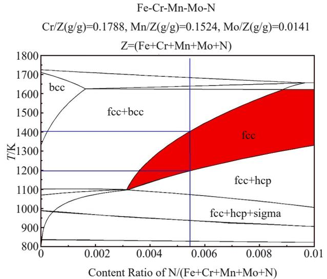
Fig.2 Phase diagram of test steel
