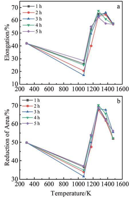
Fig.8 Elongation (a) and reduction of area (b) of test steels after solution treatment at different temperatures
