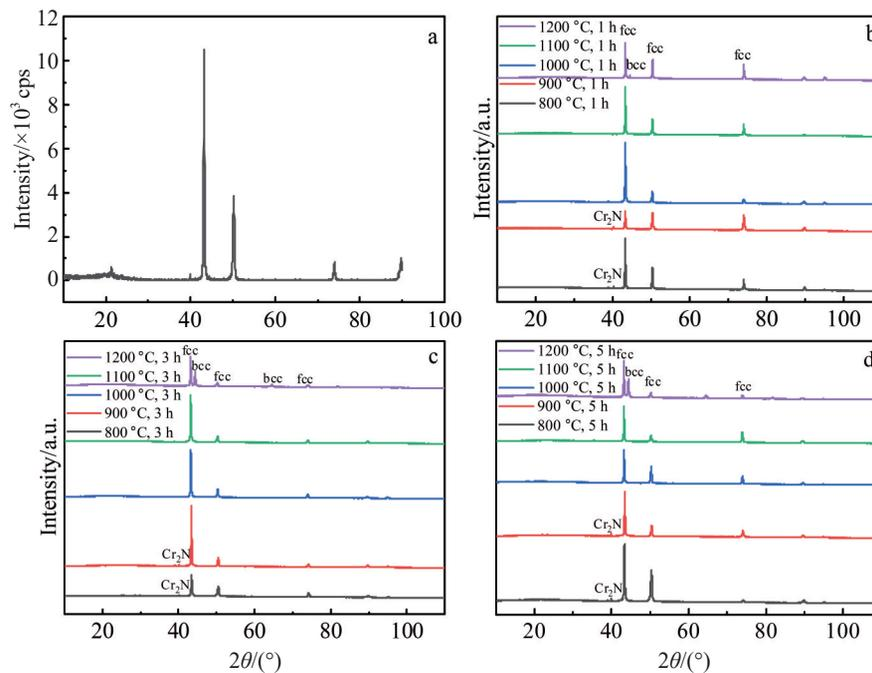
Fig.3 XRD patterns of test steels held at room temperature (a) and 800, 900, 1000, 1100 and 1200 °C for 1 (b), 3 (c), and 5 h (d)
