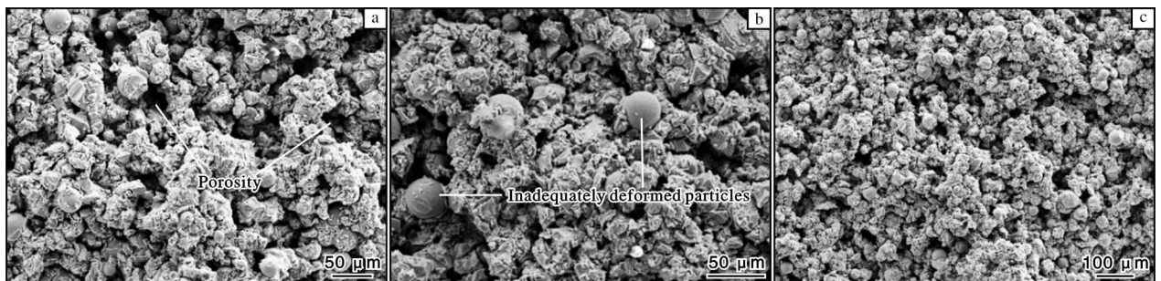
图 3 不同温度下冷喷涂 TC4 涂层试样的表面微观形貌 Fig. 3 Surface micro-morphologies of specimens cold sprayed TC4 coating at different temperatures: (a) 400 °C; (b) 500 °C; (c) 600 °C
