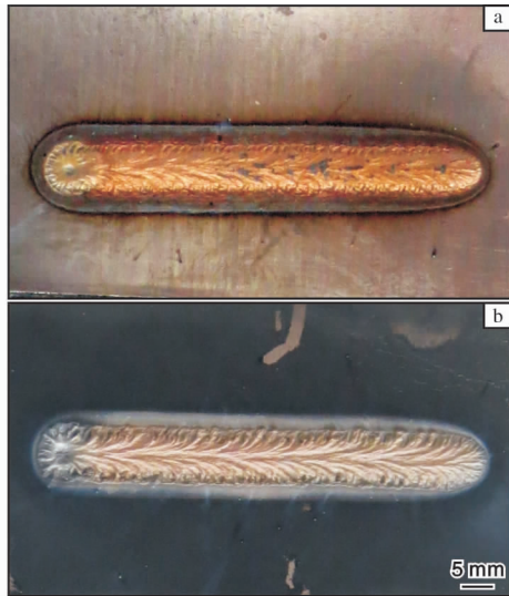
图 3 未涂覆和涂覆碳纳米管的 TC4 钛合金焊缝外观形貌 Fig. 3 Weld appearance morphologies of TC4 titanium alloy: (a) without carbon nanotubes; (b) with carbon nanotubes
